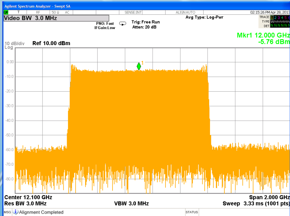
Fig. 2 - 1 GHz Modulation Spectrum using a Triangle signal
