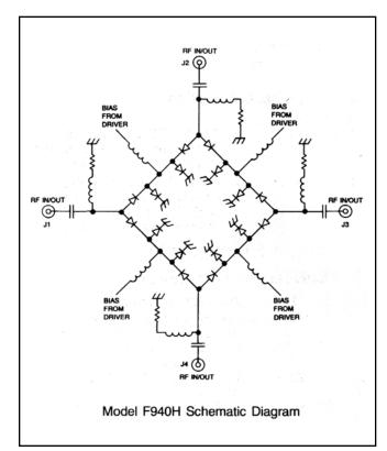
The Model F940H is equipped with an integrated driver that is powered by +5 and -12 volt supplies. The proper currents required to switch the ports ON or OFF are provided by the driver, which is controlled by external logic signals.
