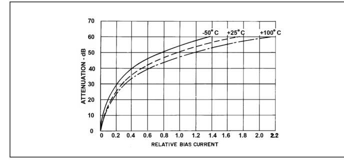
Fig 3-Series 195, typical effects of temperature on attenuation
