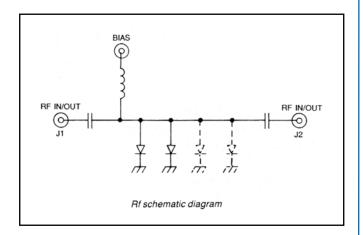
Application of a positive current to the bias terminal switches the unit OFF since the diodes are biased to a low resistance value. With zero or negative voltage at the bias terminal, the diodes are biased to high resistances and the unit is switched ON. Maximum rise and fall times are less than 10 nsec.
