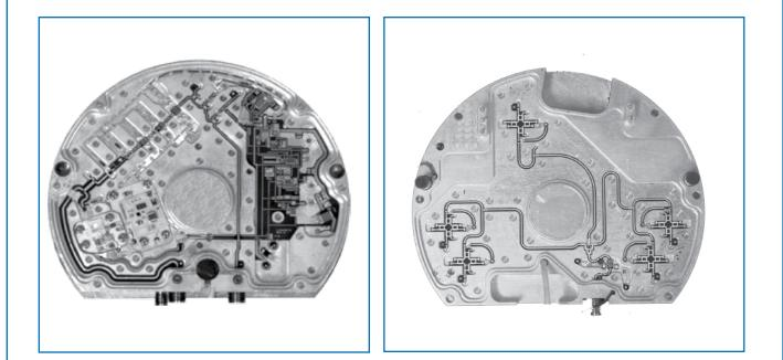
Fig. 3 - Millimeter Wave Transmitter Assembly
