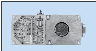
Fig. 1 - Multi-Band DTO (RF side view)
