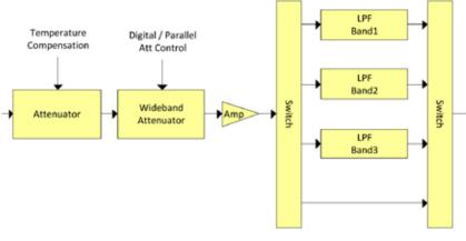
Figure 1: Amplitude Control Module Block Diagram
