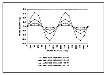
FIGURE 3 Phase Error Due to Amplitude Imbalance
