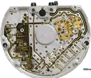
Millimeter Wave Transmitter Sub Assembly
