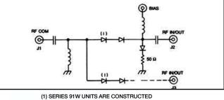
WITH THREE SERIES DIODES Series 91T, 92T and 91W schematic diagram
