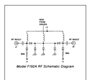
The currents required to switch the unit ON or OFF and simultaneously maintain a bilateral 50-ohm impedance match in both states are provided by the integrated driver, which is controlled by an external logic signal.
