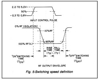
Fall Time is the time between the 90% and 10% points of the square-law detected RF power when the unit is switched from full ON to full OFF.
