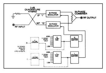
FIGURE 4 Series 71/71 Block Diagram
