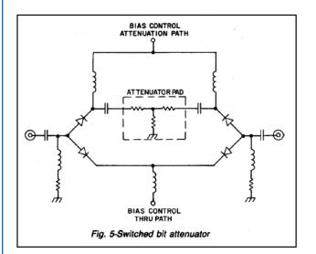
about 0.5 dB due to interacting VSWR's as the bits are switched. These interactions may lead to a nonmonotonic response as the attenuation is changed in increments of one LSB, i.e., the attenuation level may actually decrease when an increasing attenuation step is called for. Second, because of the RF circuit complexity, the cost of this attenuator is usually higher than other approaches. Finally, the incorporation of high speed switches may lead to excess video leakage.
