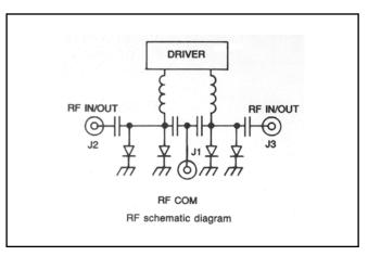
The proper currents required to switch ports ON or OFF are provided by the integrated drivers which are controlled by external logic signals.
