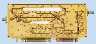
Model ACM2218 2 to 18 GHz Amplitude Control Module
