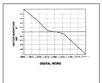
FIG. 2 TYPICAL IQ CONTROL CHARACTERISTICS
