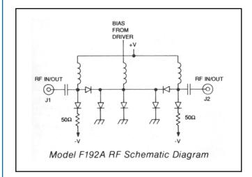
The currents required to switch the unit ON or OFF and simultaneously maintain a bilateral 50-ohm impedance match in both states are provided by the integrated driver, which is controlled by an external logic signal.
