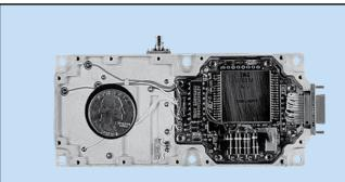
Fig. 2 - Multi-Band DTO (Driver side view)
