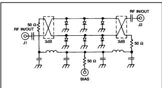
Fig. 1–Model 1959, RF schematic diagram
