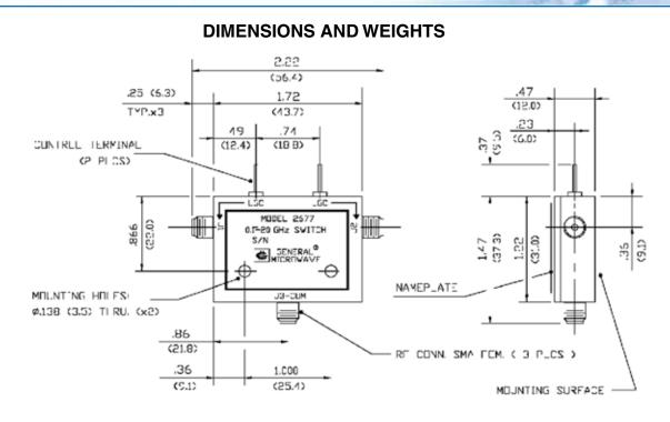
1. DIMENSIONS IN ( ), ARE IN MILLIMETERS
